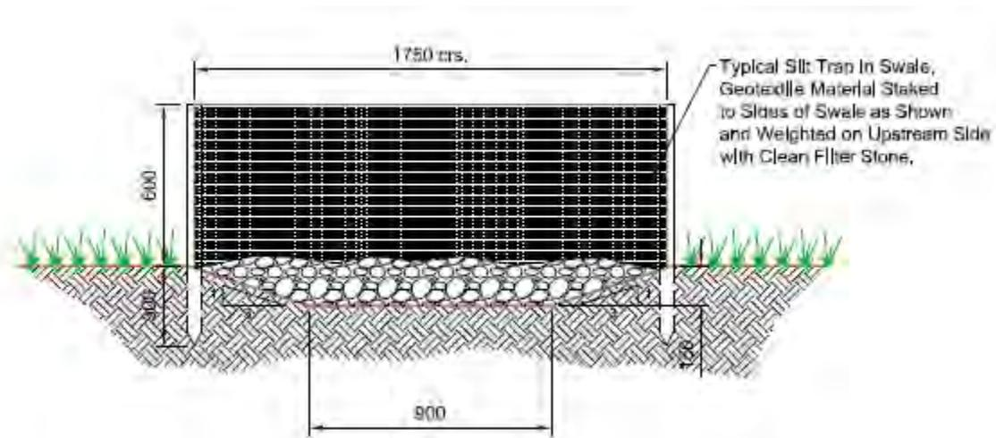
Figure 4-6: Silt Trap Details
