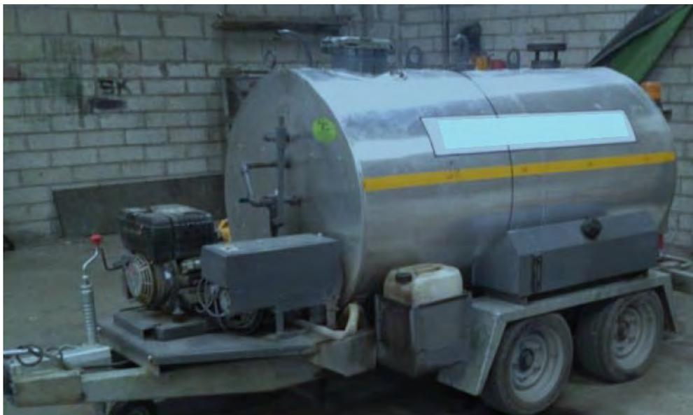
**Plate 3-7: Towable Sprayer for Temporary Reinstatement**
