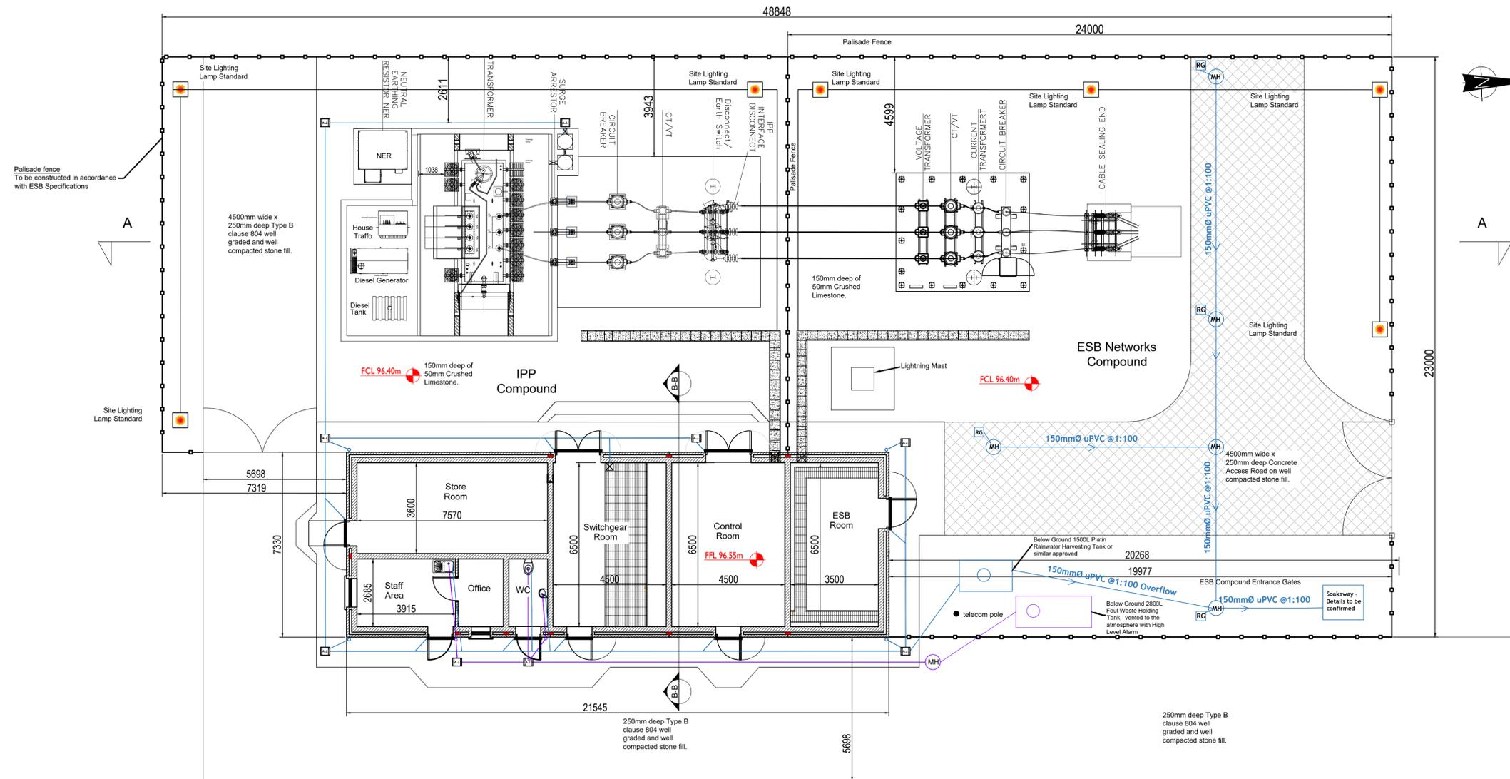
**Solar Farm-Substation Compound Layout**
