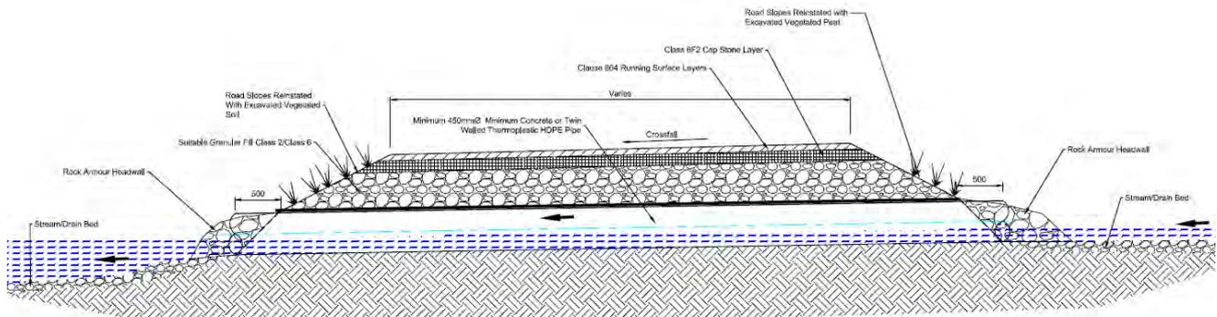
**Plate 3-1: Piped Culvert Crossing Long Section**
