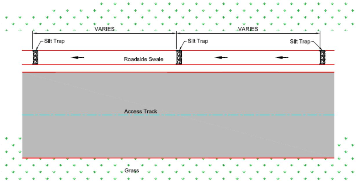
Figure 4-5: Plan of Silt Trap in Swale
