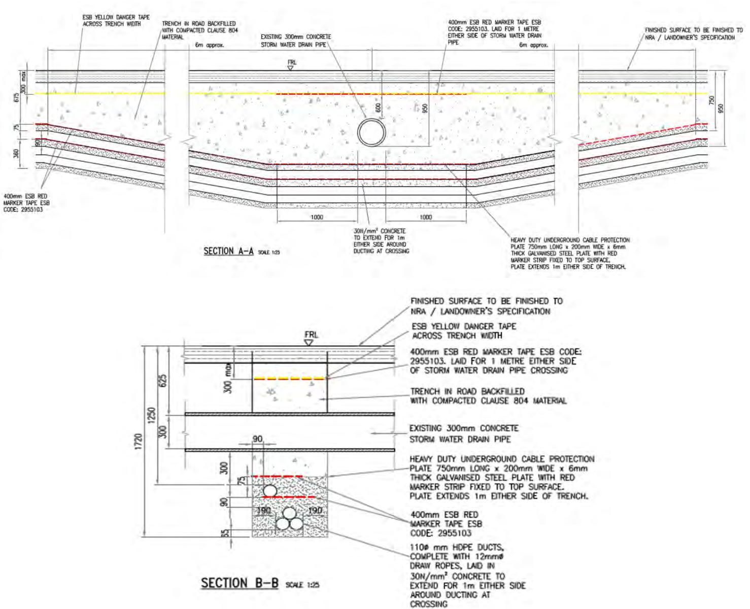
**Plate 3-4: Piped Culvert Crossings - Ducting under Culvert Crossing Details**
