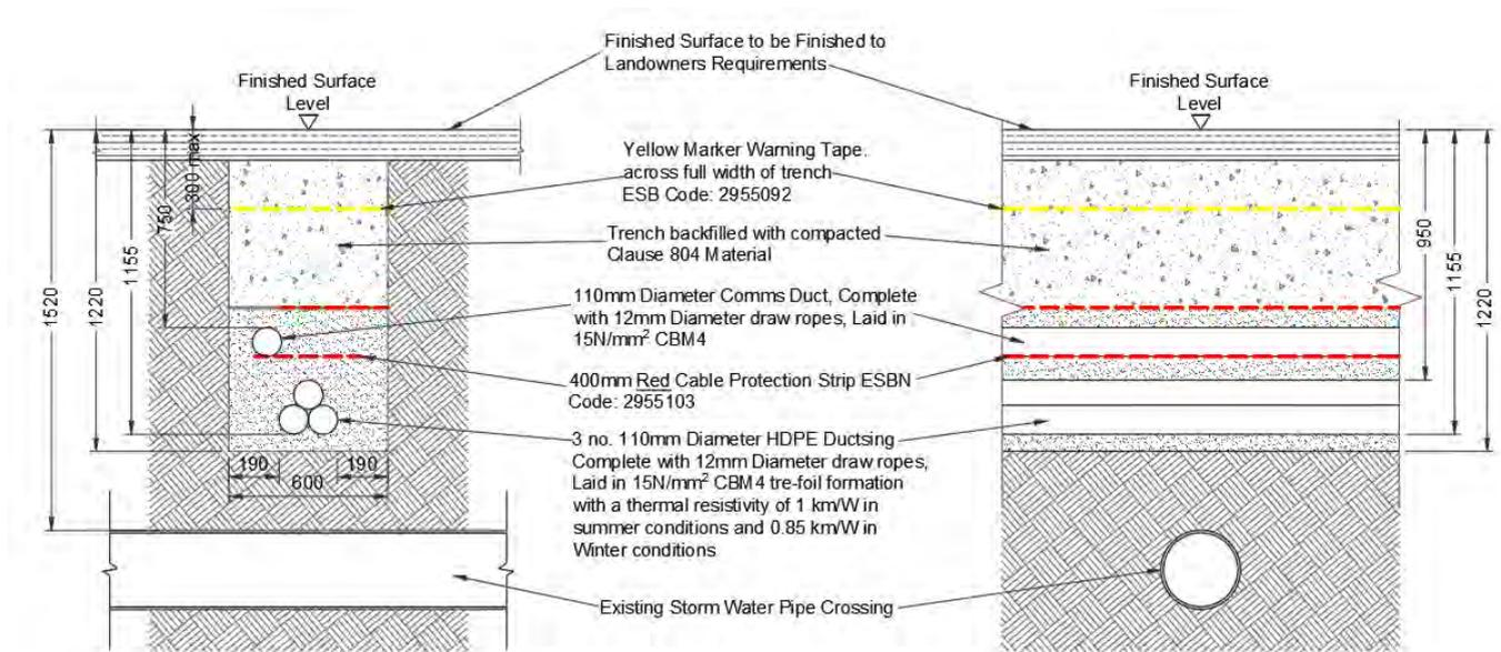
**Plate 3-3: Piped Culvert Crossing – Ducting Over Culvert Crossing Details**
